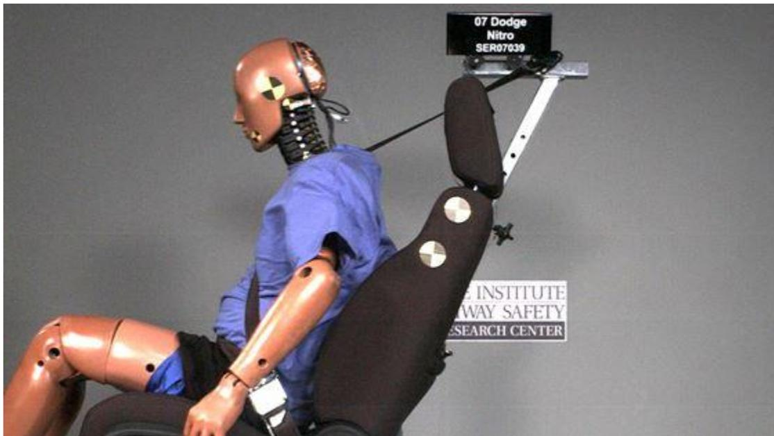
The Institute has been measuring and rating head restraint geometry since 1995. The higher and closer a restraint is, the more likely it will be to prevent neck injury in a rear collision. The Institute added a dynamic test simulating a
