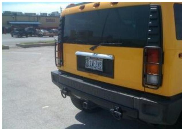
The change of velocity (delta V) experienced by the Hummer (Figures F, G, and H) was not the same as its occupant. It appears that the Hummer has very little damage but the occupant can experience high acceleration. The fact the Hummer has a trailer hitch induces a 22% increase in the acceleration pulse.
