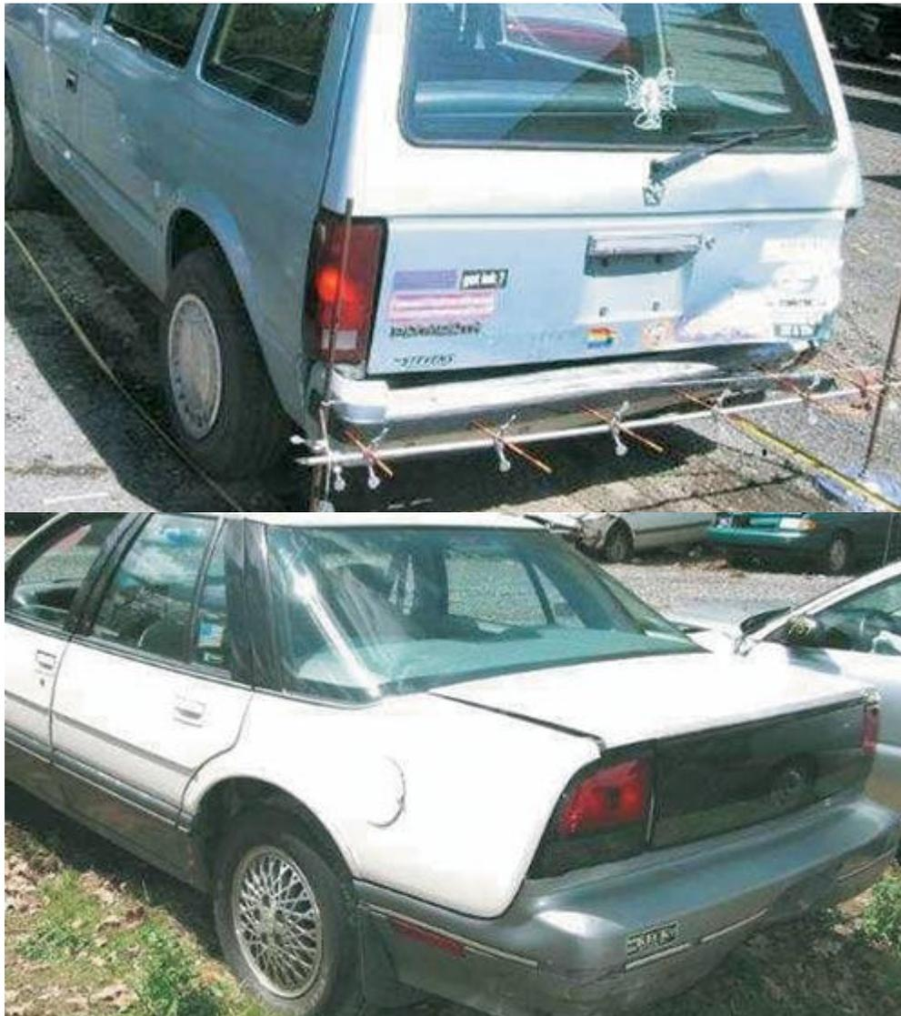
These vehicles didn't sustain a lot of damage when they were struck from behind, but the drivers were treated for injuries suffered in the impacts. Neck sprains and strains are the most serious problems reported in about 1 of 3 insurance claims for injuries. This
