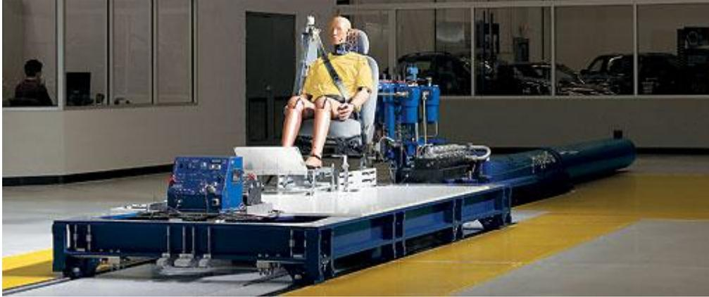
A BioRID dummy is used in dynamic sled testing, which simulates rear impacts.
